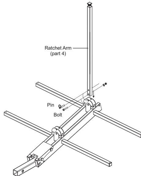
**INSTALLING THE XTC4 ONTO YOUR VEHICLE:**
